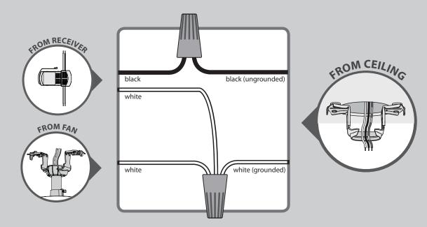
CONNECT WIRES FROM RECEIVER AND FAN TO WIRES FROM OUTLET BOX - Using the orange wire connectors, connect the black wire (ungrounded) from the ceiling to the black wire from the receiver. Connect the white wire (grounded) from the ceiling to both the white wire from the receiver and the white wire from the fan.
